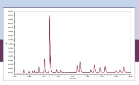
The exceptional flow rate and injection precision of the Altus UPLC $^{\circ}$  is demonstrated by the chromatographic overlay shown above – 10 gradient runs of a 19 PAH standard mixture.
