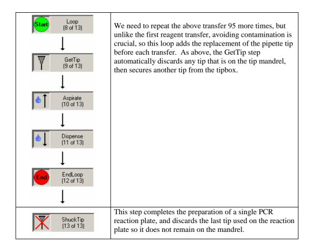
The PCR reaction plate can now be removed from the SOLO and is ready, after sealing, for the thermocycler.
