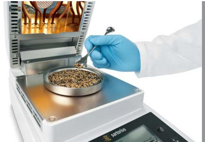
Lab Weighing | MA35 Moisture Analyzer
