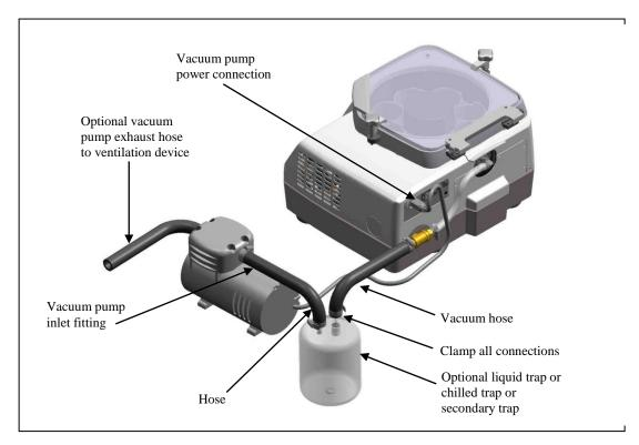
There is a switch on the back of the RapidVap Vacuum that is used to select the operation of an optional RapidVap Trapping Valve. When the RapidVap is used without the Trapping Valve as shown above, set the switch to the "Off" position.
