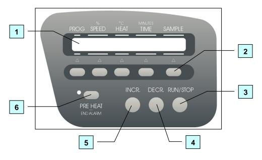
1. Display – The liquid crystal display (LCD) shows set point parameters and actual measured conditions.
