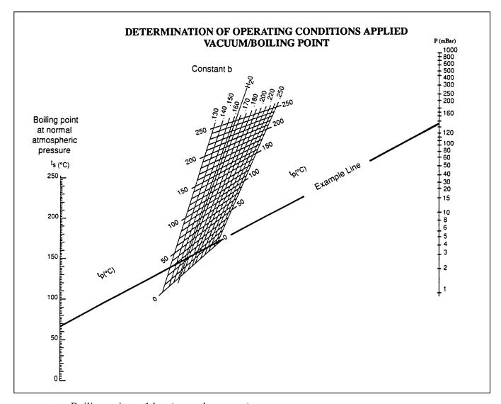
$t_s$  = Boiling point at 1 bar (normal pressure)
