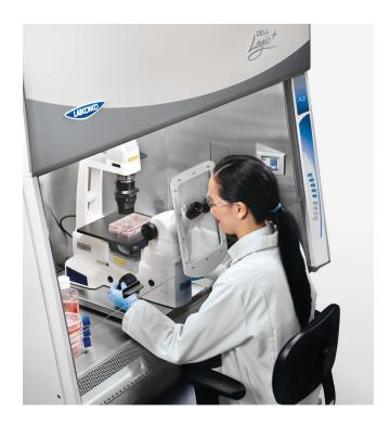
**Scope-Ready**<sup>™</sup> **Package.** Enhances comfort and performance when using a microscope in the cabinet.
