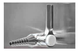
Service Fixture. Ball-type valve supplies water, vacuum, air or noble gases to cabinet interior. Serrated tip with quarter turn handle is mounted 8.5" (20 cm) above the work surface to maximize usable surface area. Max 40 psi. Accessory Package includes one right-hand service fixture (3', 4', and 5' models) or one service fixture on each side (6' models).
