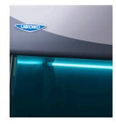
**UV Lamp.** For secondary decontamination while cabinet is not in use. Safety switch permits operation only when sash is completely closed. 254 nm.
