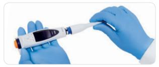
1. Unscrew the tip ejector collar counter clockwise and remove it. Remove the Safe-Cone Filter if fitted.
