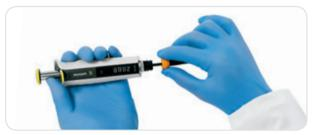
2. Unscrew the tip cone holder counter clockwise and carefully remove it along with the tip cone.
