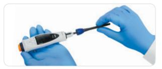
2. Unscrew the tip cone holder counter clockwise and carefully remove the tip cone holder, tip cone and spring.
