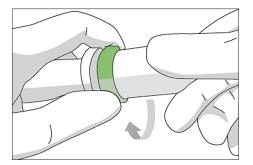
c. With a 10 ml pipette hold the tip cone cylinder firmly and turn the locking ring (2) clockwise with your fingers (see image below). Do not turn the tip cone (3) as this will break the pipette.
