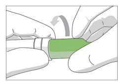
b. With a 5000  $\mu$ l pipette, hold the locking ring (2) firmly with your fingers and turn the tip cone cylinder counterclockwise with the other hand (see image below). Do not turn the locking ring as you turn the tip cone (3) as this will break the pipette.
