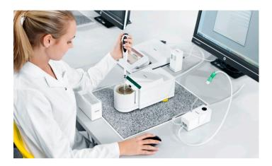
For some electronic pipettes, such as Sartorius Picus<sup>®</sup> Nxt, the calibration interval can be set by activating the calibration reminder. The function will notify you when the previous calibration is about to expire. You can also lock the Sartorius Picus<sup>®</sup> Nxt pipette if you suspect that the pipette is not working properly; this prevents others from using the pipette until it has been checked.
