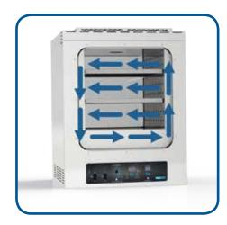
The SHEL LAB high volume blower system circulates air through stainless steel air ducts, providing horizontal one pass airflow. This horizontal airflow provides superior temperature uniformity and fast heat-up capabilities. The unique air ducts move heated air and direct it to the right side of the chamber. Our precise horizontal airflow delivers performance even under maximum capacity oven loads.
