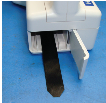
Figure 3-2 Pull Battery Release Ribbon Out
