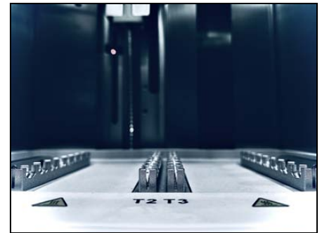
Heating strips for lysis & elution
