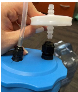
Figure 1: HEPA filter placement and EVA tube attachment for a single unit setup
