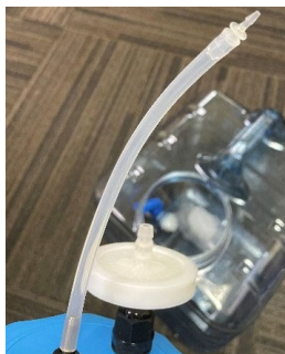
Figure 1: HEPA filter placement and EVA tube attachment for a single unit setup
