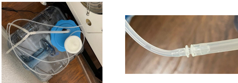
Figure 5: Thin tubing from incubator shaker connected to carboy via 2-way connector
