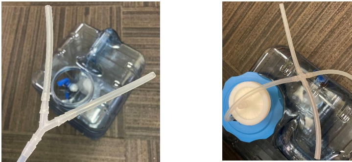
Figure 2: EVA tubing connections for a double stack (left) and triple stack (right)
