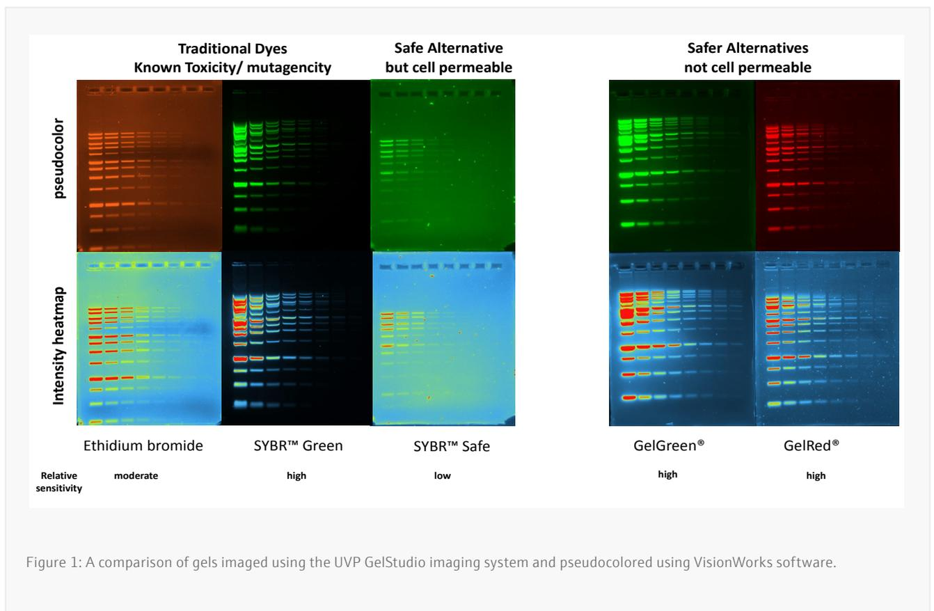
Figure 1: A comparison of gels imaged using the UVP GelStudio imaging system and pseudocolored using VisionWorks software.
