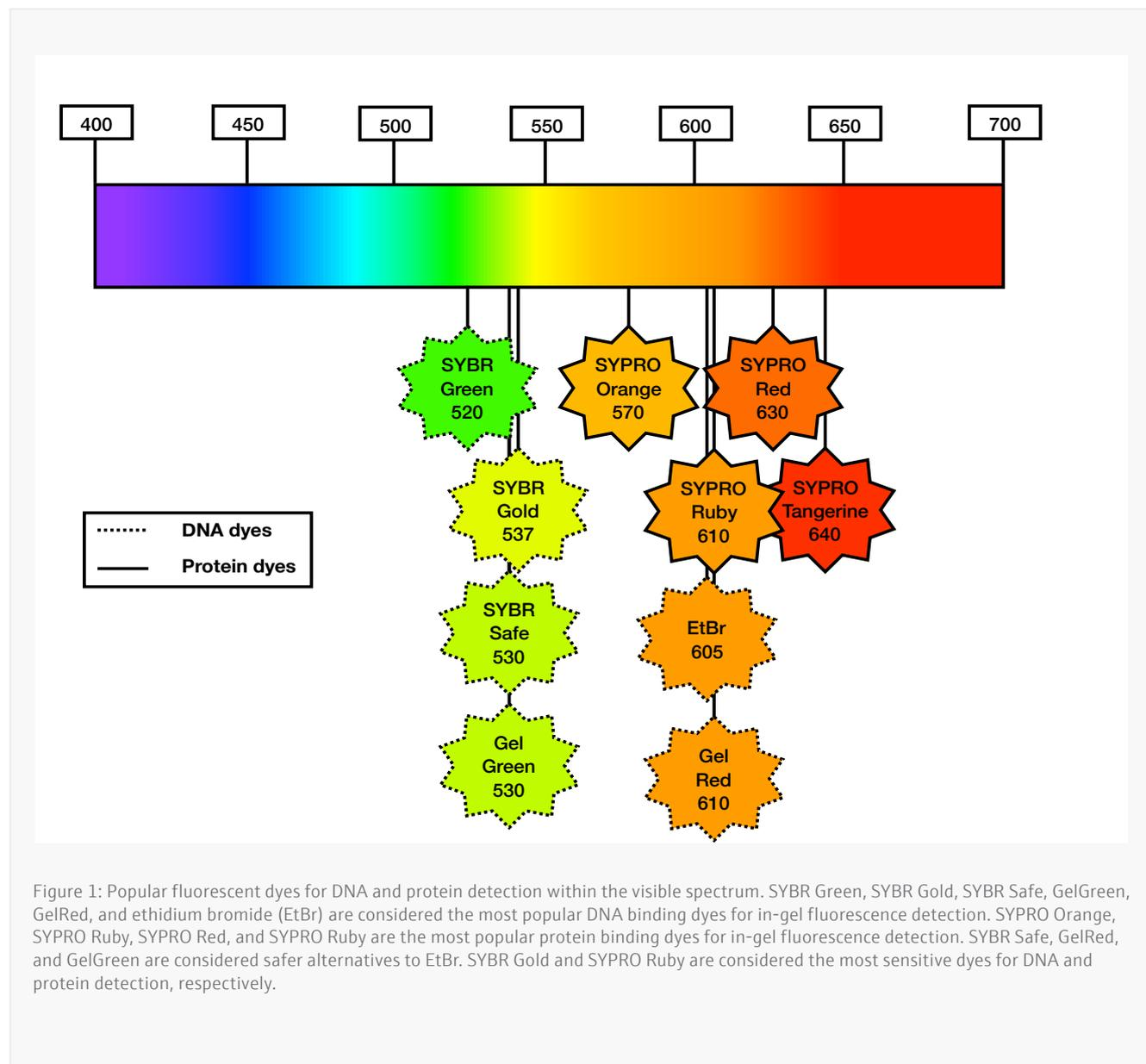
At Analytik Jena, we have designed our instruments to accommodate technologies both old and new. Importantly, all our instruments are capable of imaging gels stained with the most popular fluorescent dyes on the market (Table 1). These include safer DNA dyes like GelRed, GelGreen, and SYBR safe as well as high sensitivity SYBR Gold and SYPRO Ruby for DNA and protein detection, respectively. Below we demonstrate the diversity of dyes that can be captured with our imagers.
