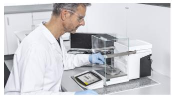
**Figure 1:** Determining the minimum sample weight on a Cubis® II MCA66S according to USP Chapter 41.
