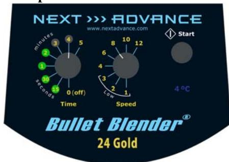
The figure above shows the Bullet Blender Gold set to run for 4 minutes at a speed of 8, after running for 2 minutes. To operate, press the "START" button. After 15 seconds, the LED light by the number 15 will light up. After 30 seconds, the second LED light by the number 30 will light up. And so on. At the settings shown above, after 4 minutes, the Bullet Blender Gold will stop.
