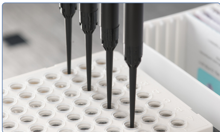
Figure 1: STAR Line robot pipetting into a PCR plate with 50µl disposable conductive tips on the CO-RE 1000µl channels.
