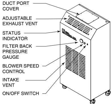
The WhisperFlow® portable HEPA filtration system is a mobile, self-contained, hospital air purifier designed to easily convert any room to a negative pressure isolation room to meet OSHA and CDC TB guidelines.
