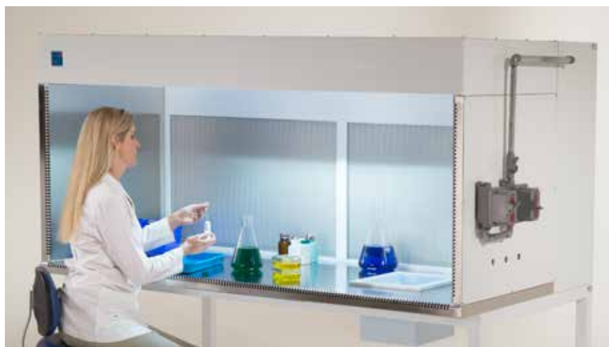
Horizontal flow model 1686-98 showing wiring encased in filled rigid conduit terminating at power switches for lighting and rear-mounted fan/filter units. Visible along front and side edges are return air ducts that reduce backflow turbulence.
