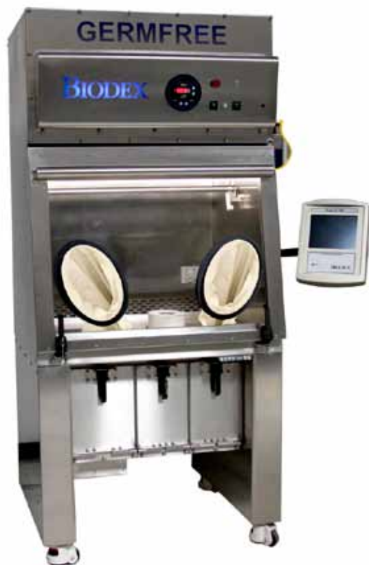
34" work area. Compounding Aseptic Containment Isolator (CACI) completely shields users from radioactive material
