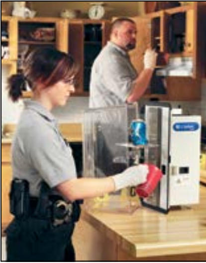
The CAPture Portable Fuming System identifies latent fingerprints on the scene and fixes them for safe transport to the laboratory.
