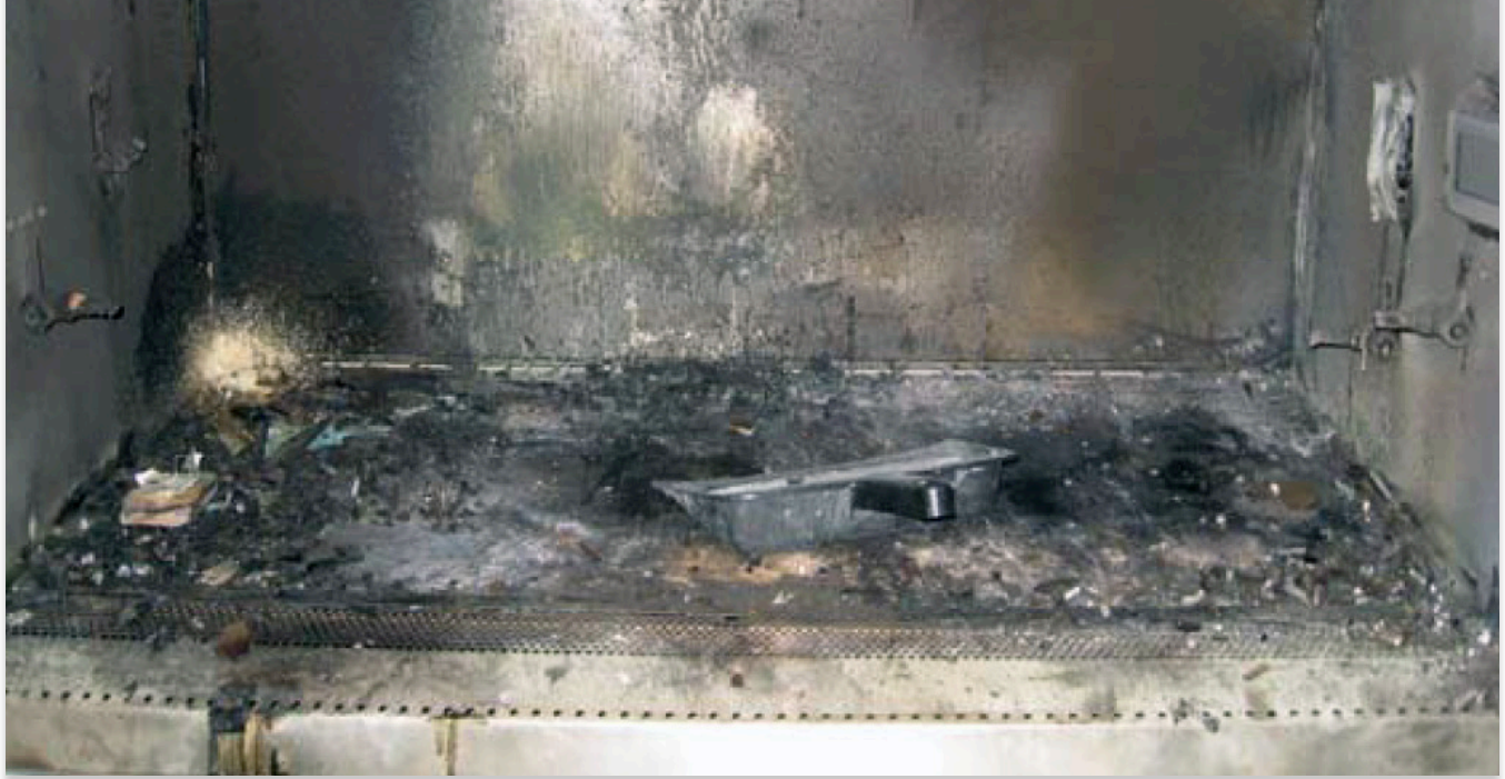
BSC with fire damage
